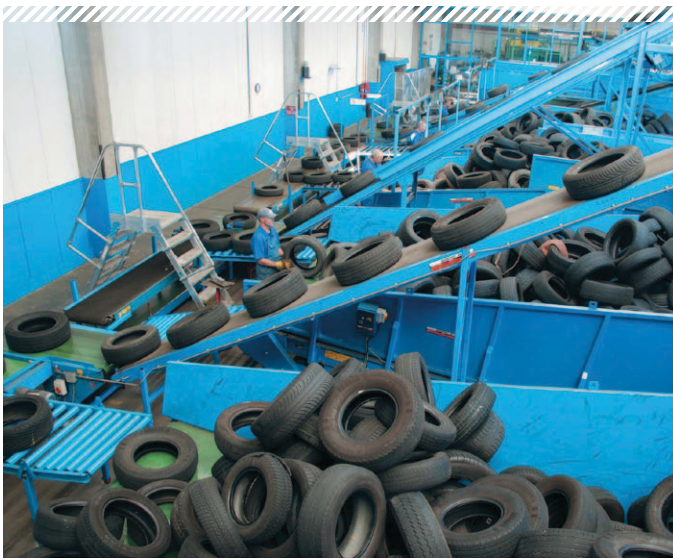
Sorting centre with the capacity to sort 10,000 tyres a day (Source: Lintire)
